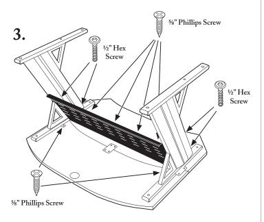
Attach the modesty panel to both legs using the ½" hex screws (4x). Tighten fully. Then install the %" Phillips screws (2x), attaching the modesty panel to the desktop. Then, using the remaining %" Phillips screws (4x), attach the legs to the desktop.
