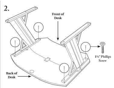
Attach the two legs to the bottom of the desk with the 1½" Phillips-head screws (4x). **Tighten screws only finger tight for now**.
