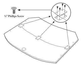
Place the two sections of the tabletop face down. Be sure to align the edge and seam so they are flush. Attach the three I-brackets using the ½" Phillips screws (12x). Tighten all the screws finger tight. Check the alignment, then tighten screws fully using a Phillips-head screwdriver.
