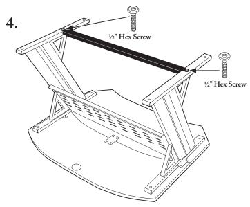
Attach the crossmember bracket to both legs using the ½" hex screws (2x). Check the alignment of the assembly, adjust if necessary, then tighten screws fully.
