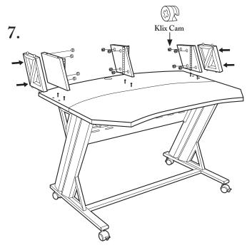
Insert Klix cams (4x) into each of the rack mount walls by doing the following: Point arrows toward the pre-drilled cam holes. Push cams into holes. Then place the decorative triangular pieces into place next to the side walls.
