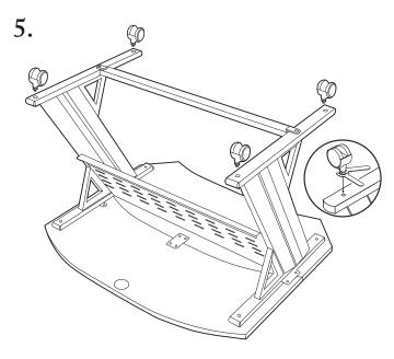
With the included Open wrenches, install the casters (4x). Position the brake-equipped casters on the "front" of the desk. Please note that these wheels are height adjustable, enabling you to match the height of the desk with other furniture.
