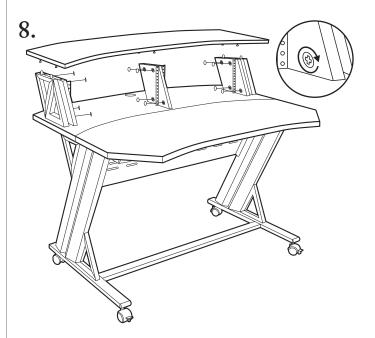
Place the desk shelf on top of the rack mount walls and tighten the Klix cams clockwise using a Phillips-head screwdriver. Use caution not to over-tighten Klix cams. To complete the assembly, place the cam covers (12x) into place.
