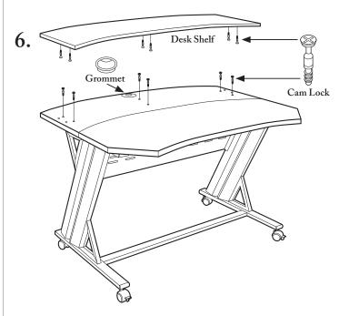
With the help of a friend, turn the desk up on its wheels. Install the cable management port grommet. Then install the cam locks (6x) into the desktop. Install the rest of the cam lock screws (6x) into the bottom of the desk shelf.
