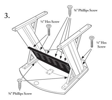
Attach the modesty panel to both legs using the ½" hex screws (4x). Tighten fully. Then install the %" Phillips screws (2x), attaching the modesty panel to the desktop. Then, using the remaining %" Phillips screws (4x), attach the legs to the desktop.
