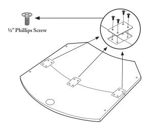
Place the two sections of the tabletop face down. Be sure to align the edge and seam so they are flush. Attach the three I-brackets using the ½" Phillips screws (12x). Tighten all the screws finger tight. Check the alignment, then tighten screws fully using a Phillips-head screwdriver.
