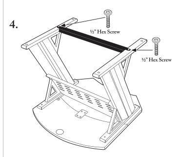
Attach the crossmember bracket to both legs using the ½" hex screws (2x). Check the alignment of the assembly, adjust if necessary, **then tighten screws fully**.
