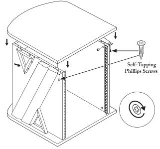
To attach the top panel, first attach the top decorative triangles to the metal posts by sliding them into position, nub to hole. Then place the remaining Klix cams (4x) in the appropriate holes. Make sure all connecting hardware are in the right position and aligned correctly. Tighten cam locks fully. Then install self-tapping Phillips screws (2x).
