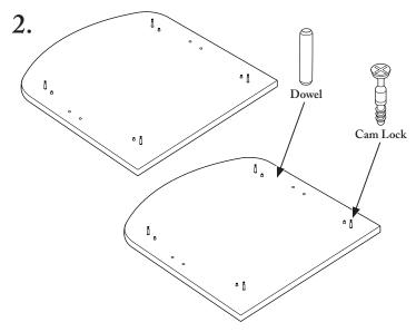
Install cam locks (4x) and dowels (4x) on the underside of the top panel. Then, install cam locks (4x) and dowels (4x) on the topside of the bottom panel.
