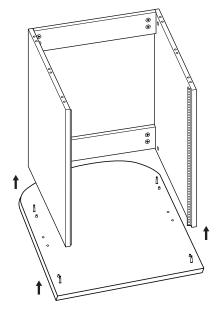
To attach the bottom panel to the side panels, install the Klix cams (4x) to the bottom holes of the side panels. When all the connecting hardware are in the right position and aligned correctly, attach the bottom panel. Then, install tighten the Klix cams with a Phillips-head screwdriver.
