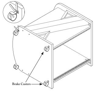
Turn the unit sideways again. With the included open wrenches, install the casters (4x). Make sure the "brake" casters are placed at the front of the unit. Also, please note that these wheels are height adjustable, enabling you to match the height of the sidecar with other furniture.
