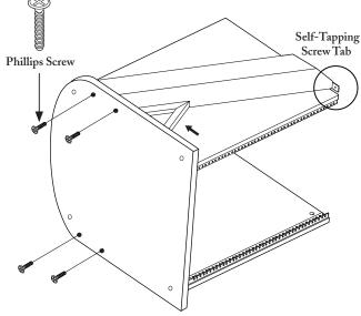
Turn the unit sideways with the bottom panel facing toward you and attach the metal posts (2x) by inserting Phillipshead screws (4x) through the underside of the bottom panel. Make sure the self-tapping screw tap is positioned as shown in illustration. Repeat for the other side. Attach the bottom decorative triangles by sliding into position, nub to hole.
