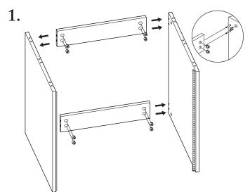
Install Klix cams (4x) to each of the rear support panels. Then, install cam locks (4x) into each side panel. Attach side panels to rear supports and tighten cam locks with a Phillips-head screw driver.
